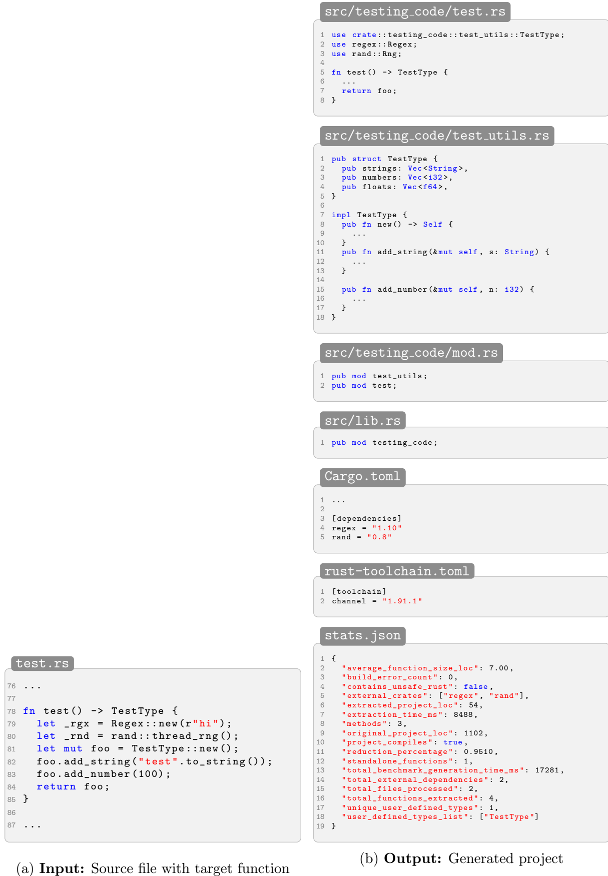
Figure 4.2: Full extraction example of target function test . The left panel shows the original source code file containing the target function. The right panel shows all extracted files.
